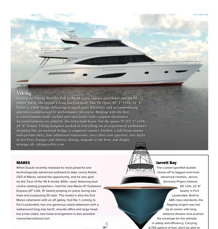
go far and fast with 2,600-hp 16-cylinder MTUs that propel her into the mid-30s. Lightweight construction helps in this endeavor: carbon fiber stringers and bulkheads, titanium shafts and ultra-thin marble veneer flooring. Six staterooms are incorporated, including a full-beam master and two separate crew quarters, and the finish throughout is impeccable.
