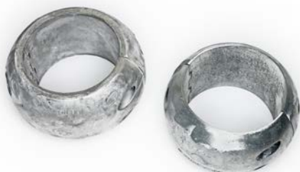
aluminium (left) can easily be mistaken for zinc (right)
